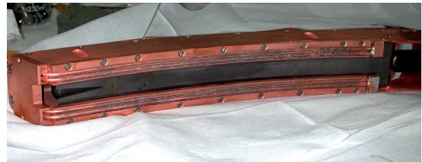
Figure 6: Deflector with cooling circuit in contact with the septum
